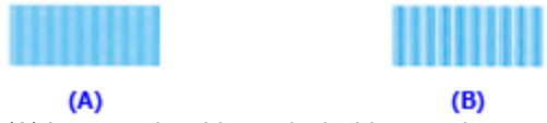
(A) Least noticeable vertical white streaks (B) Most noticeable vertical white streaks
